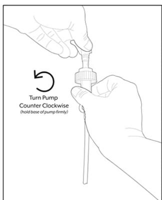
Hold the base of the pump mechanism just below the cap with your right hand and grasp the pump head with your left hand.
